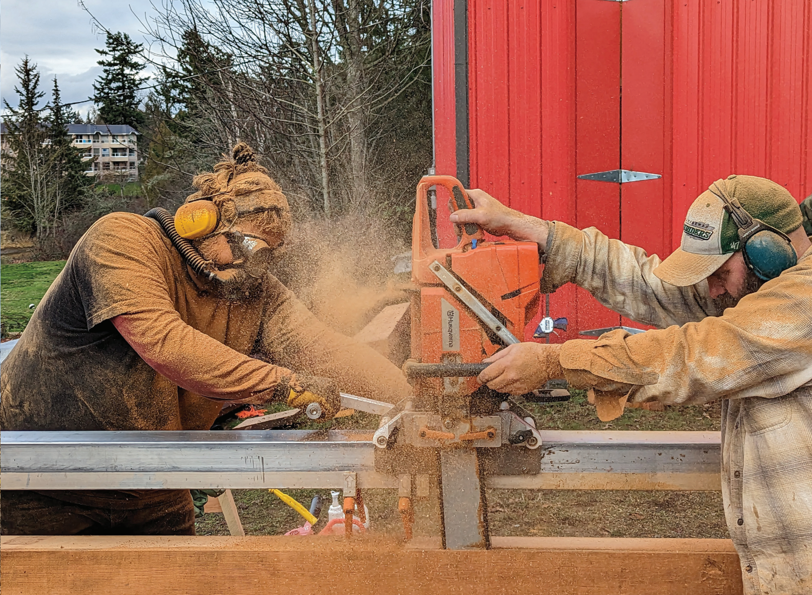
Tejas Collinson (L) and Colin Graham use the chainsaw milling attachment of the Totem 2.0 device to cut the raw timbers down to size.
