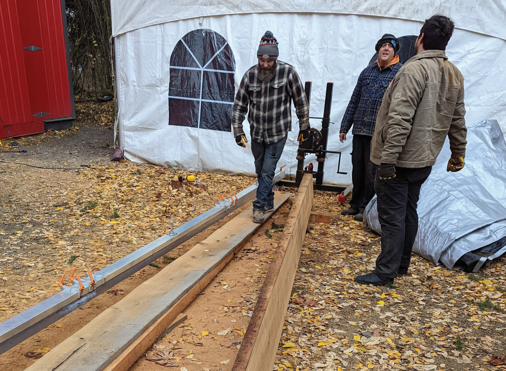
(L to R) Colin Graham, Carey Newman, and Tejas Collinson prepare to remove the milled timber from the Totem 2.0 device.
