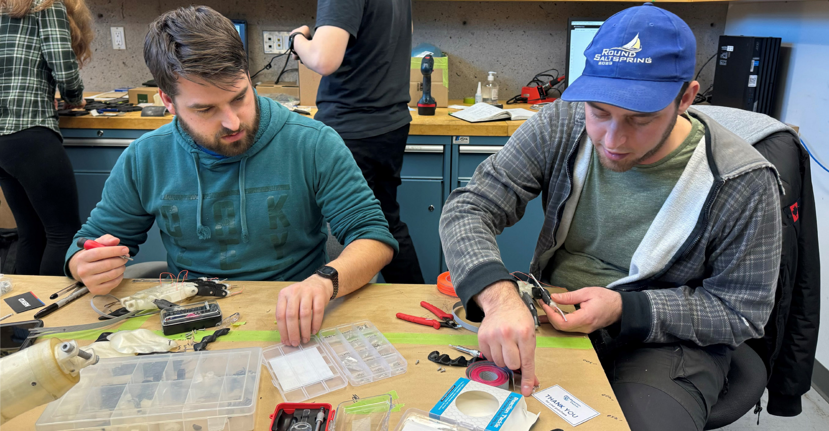
Luke Rosenberg and James Skittrell work on assembly of the hand tendons, springs, and sensor conduits.
