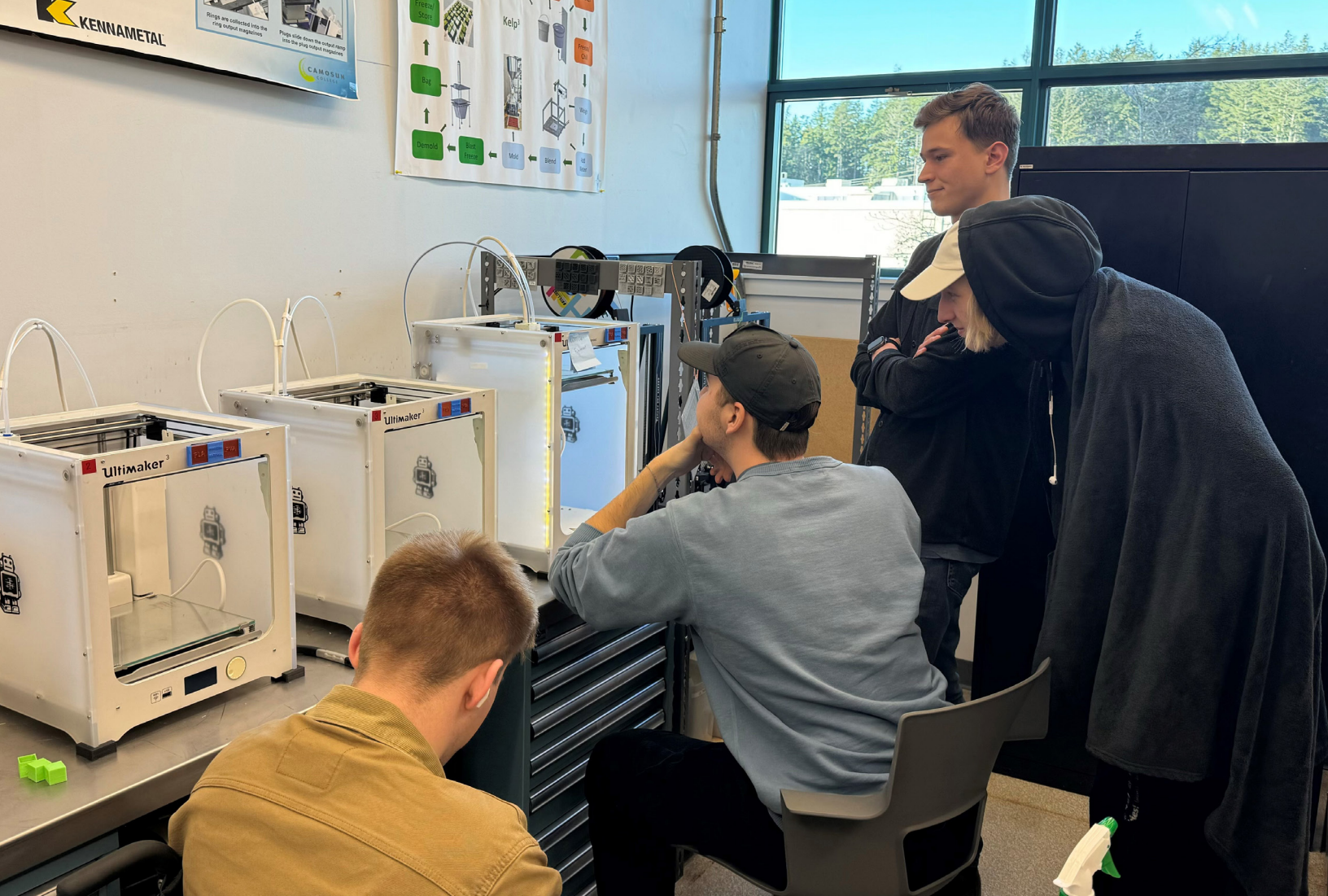
Sam Valensky, Jeremy Turmel, Dylan Snyder, and Matthias Wegner supervise the first few layers of a 3D print to make sure there is proper adhesion to the bed and no clogged printing nozzles.
